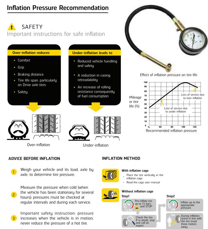
Pressure gauges: must be accurate, handled with care and calibrated regularly
